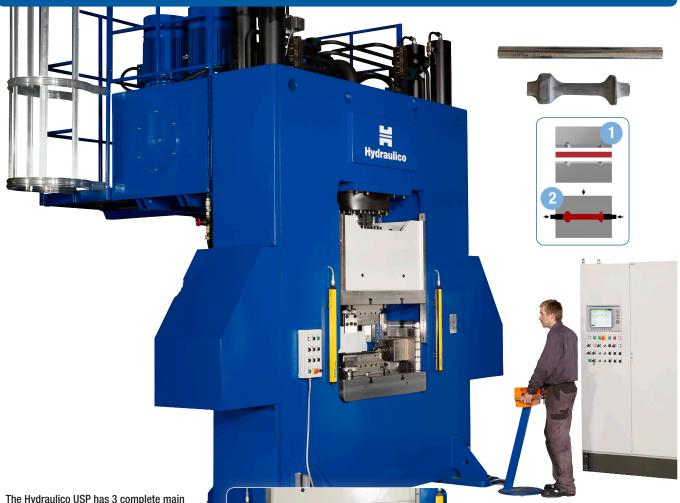
The Hydraulico USP has 3 complete main systems: one clamping cylinder (A) and two side forging cylinders (B) and (C).
